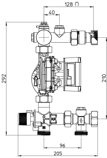
(\*) the dimension is the same even for the model with 1" Male connection to the manifold
